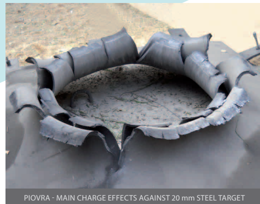
PIOVRA - MAIN CHARGE EFFECTS AGAINST 20 mm STEEL TARGET
